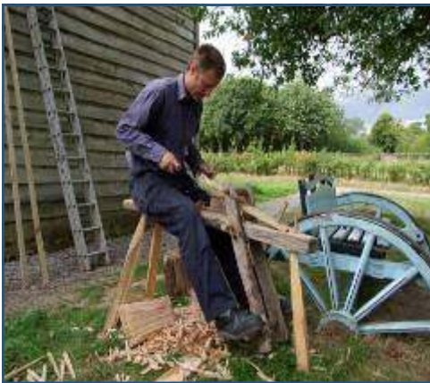
Joe making wooden pegs on a shaving horse to peg the door frame together
